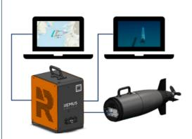
Odyssey Sim components can seamlessly transition between software and hardware-in-the-loop operation modes. This capability allows for wide system test coverage in virtual operational environments before sea trials and enables customers to plug in 3rd party autonomy or payloads for rapid integration. The use of digital REMUS has led to a reduction in required test days at sea and expanded available services for REMUS customers with accurate mission verification.
