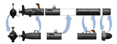
**Configuration.** Odyssey Sim is built with a modular architecture for customization and expandability of simulations. A simulated vehicle can exercise any sensors in any configuration and be deployed in a virtual environment uniquely crafted by the operator.
