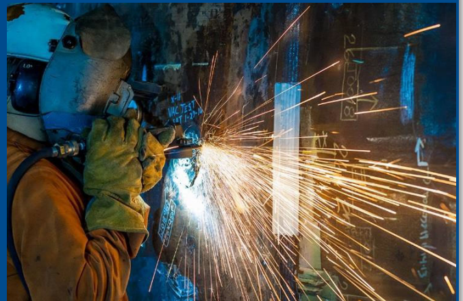
A shipbuilder cleans up welds on the Delaware SSN 791 for magnetic particle inspection. Photo by Chris Oxley.
