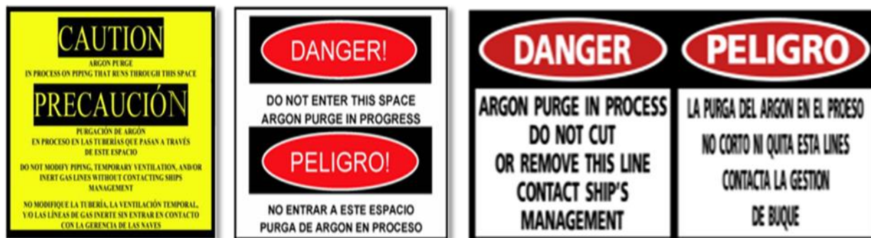
Safety signs used in communicating inert gas purging operations..
