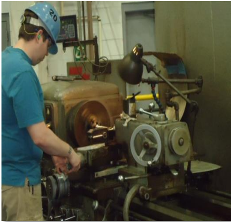
Operating lathe without chuck guard in place.
