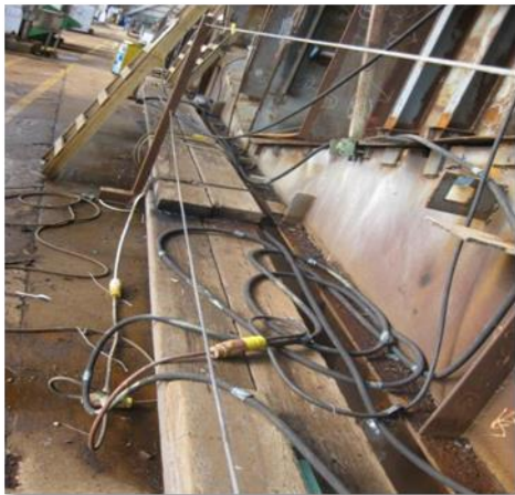
Poor line control. Walkways must be kept clear of lines. Walking on lines will damage them and create other hazards.
