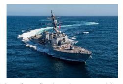
Guided missile destroyers are the backbone of the U.S. surface fleet and are capable of fighting multiple air, surface and subsurface threats simultaneously. The Flight III Arleigh Burke-class destroyers incorporate a number of design modifications that collectively provide significantly enhanced capability including the AN/SPY-6(V)1 Air and Missile Defense Radar (AMDR) and the Aegis Baseline 10 Combat System.
